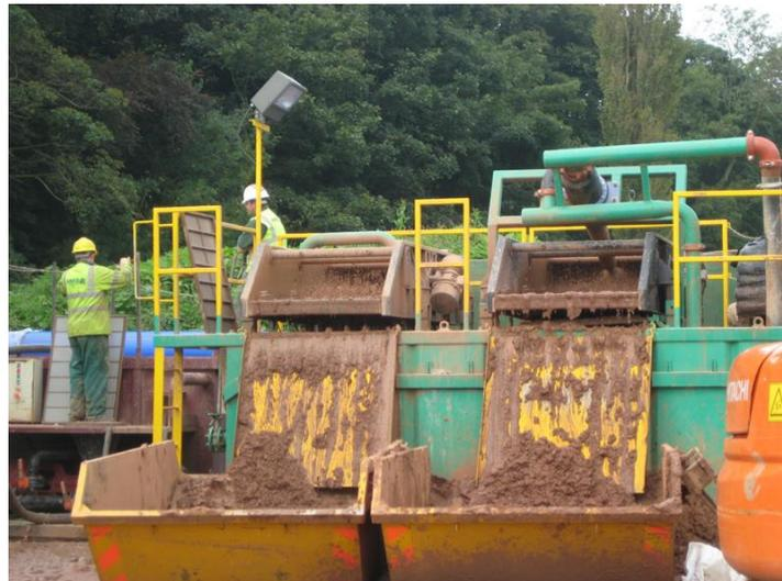
*LCC500 mud recycling unit in operation*
